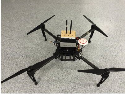
Fig. 7: Experimental Platform equipped with an Intel NUC computer, an Intel 5300 Wireless card with two antennas, and an IMU
